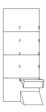
3. Starting from the bottom, hook trays into slots.
